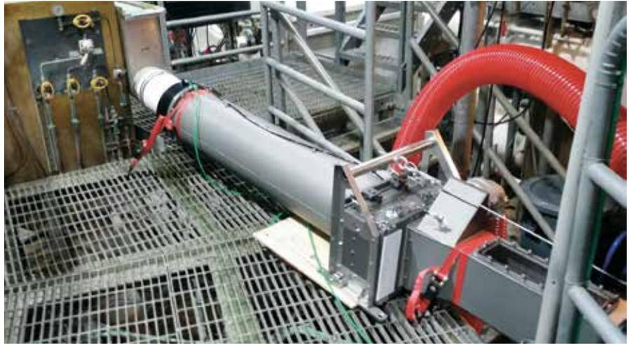
The “accelerator” is attached to the side wall drop box of a tank (left rear). Fish that enter the system are “whooshed” along via the exit at the lower right. The red tube pulls air out of the system. A second tube underneath (not shown) pushes air.
