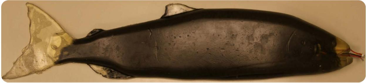
Figure 2. Silicone Fish #1 was used for all treatments. An internal Sensor Fish (Sensor Fish #56) was embedded in the silicone fish. Wires connect the internal Sensor Fish to the outside which enables data download. Two samples were collected for each treatment. Atmospheric pressure was about 14.3 psi during testing on September 20, 2015.
