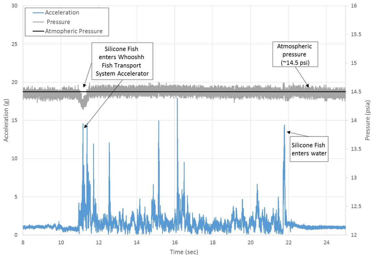
Figure 1. The instantaneous acceleration and pressures measured by the Sensor Fish as it moved into, through, and out of the Whooshh Fish Transport System (WFTS) on November 5, 2014. Entrance to the WFTS is noted by the slight increase in pressure, and exit from the WFTS is noted by the slight decrease in pressure (return to pre-passage pressure). There were peaks in the acceleration measurements as the Sensor Fish moved through the tube, the largest likely as the
