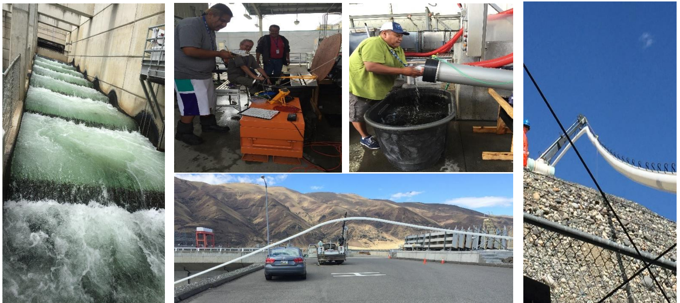
Figure 2. Images from the 2016 Priest Rapids Sockeye migration study. Left: remaining ladder climb after sampling at OLAFT. Top Left: CRITFC and Yakama Nation crew sampling and PIT tagging Sockeye at OLAFT. Top Right: Hand feeding Sockeye into the WFTS. Right: Week 30 WFTS fish transporting to top of the dam. Bottom: Week 30 WFTS spanning the dam crest.
