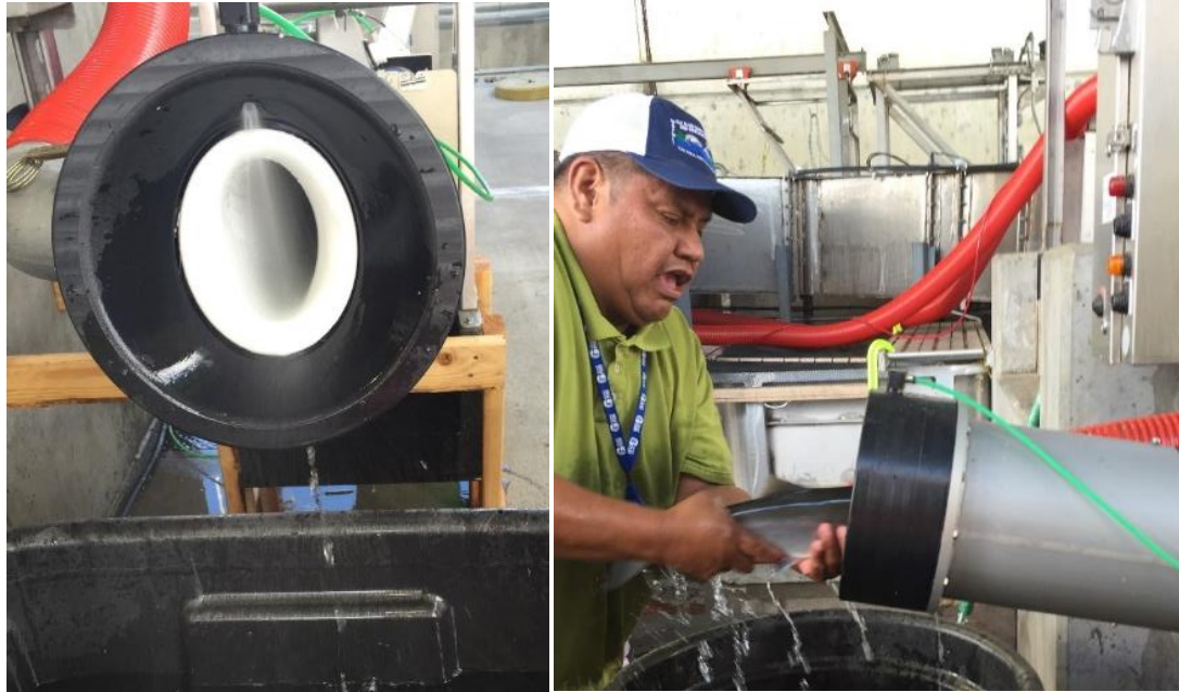
Figure 2. Left image is the entrance to the WFTS accelerator. Right image is a side view example showing a Sockeye salmon being hand fed into the T123 accelerator entrance.
