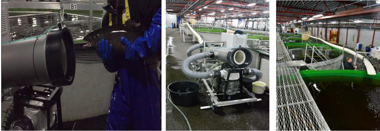
Figure 4. The WFTS set-up at AquaGen's broodstock facilities. Left photo: handloading Atlantic salmon into the WFTS. Middle photo: WFTS entry side next to the holding tank. Right photo: WFTS exit into the observation tank.
